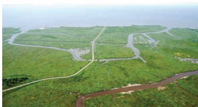
TORN SALT MARSH in Delaware Bay ( top, 1998 ) was restored by cutting a few gaps in adjacent dikes so freshwater could flow in and naturally create tidal creeks, which allowed plants to reseed and flourish ( bottom, 2013 ).
